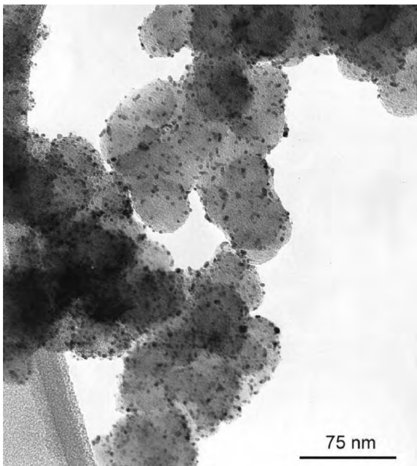
Figure 1.6 TEM image of fuel cell catalyst. The black specks are the catalyst particles finely divided over a carbon support. The structure clearly has a large surface area. (Reproduced by kind permission of Johnson Matthey Plc.)
