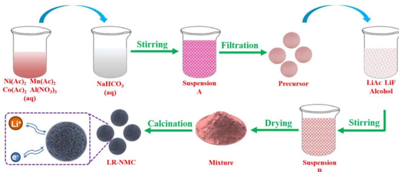
Figure 39. Schematic diagram of the preparation of precursors \text{Ni}_{0.13}\text{Co}_{0.13-x}\text{Mn}_{0.54}\text{Al}_x(\text{CO}_3)_{0.8+0.5x} and cathode materials \text{Li}_{1.2}\text{Ni}_{0.13}\text{Co}_{0.13-x}\text{Mn}_{0.54}\text{Al}_x\text{O}_{2(1-y)}\text{F}_{2y} (LR-NCM). Reprinted from [10], Copyright 2017 with permission from Elsevier.
