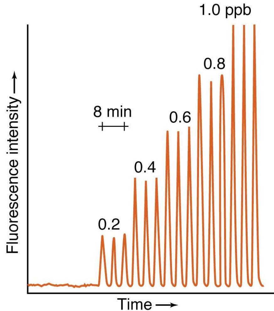
FIA of ppb levels of  $\text{H}_2\text{O}_2$  in air.
