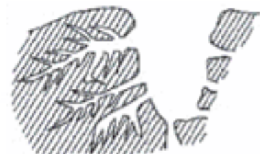
Figure 6. Schematic pore images of activated carbon fiber and activated carbon.
