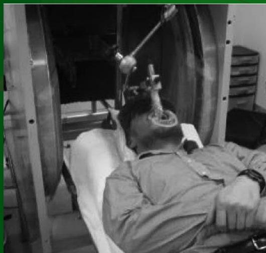
A platform to position and stabilize the foot for measurements of pO<sub>2</sub> in the foot.
