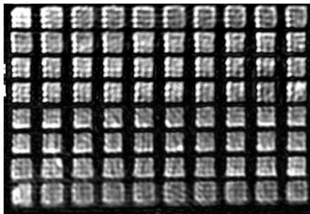
**Figure 5.** Typical image obtained with an SPR imaging sensor with a polarization control. Bright rectangles correspond to areas of an SPR chip ( $300 \times 300 \mu\text{m}$ ) covered with a monolayer of albumin molecules formed on the surface of gold by microspotting.
