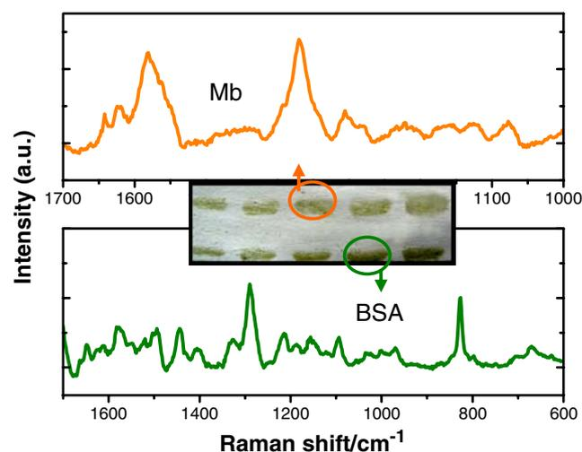
**Fig. 2** SERRS of myoglobin and SERS of BSA on an NC membrane by the proposed “Western-SERS” procedure
