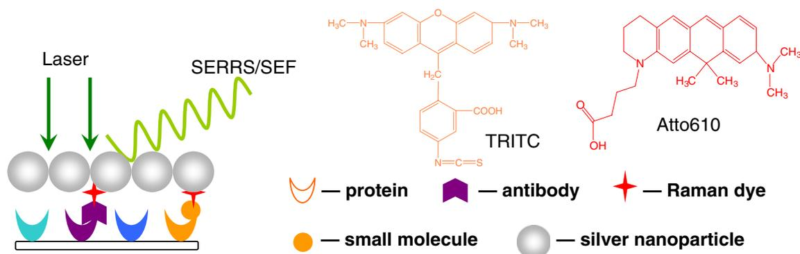
**Fig. 7** SERS-based procedure for detection of protein-ligand interactions and two Raman dyes
