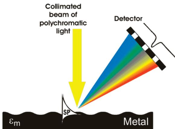
**Figure 6.** Concept of SPR sensor based on simultaneous excitation of surface plasmons by a polychromatic light and the dispersion of light on a special grating coupler.<sup>127</sup>
