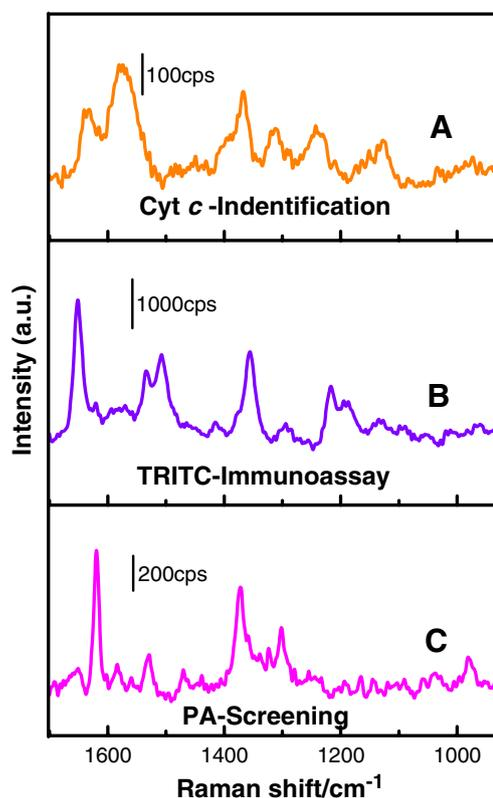
**Fig. 10** SERS of cytochrome *c*, TRITC and pipemidic acid (PA) from the Au/Ag sandwich substrate
