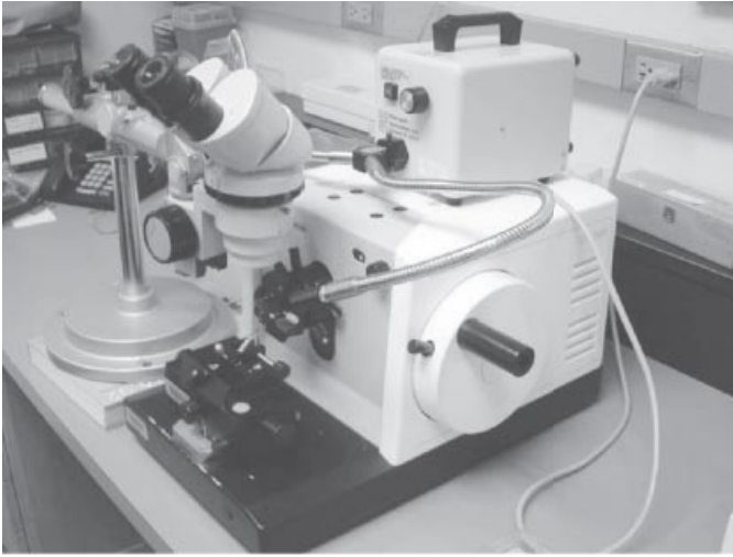
Figure 5.10 Microm manual rotary microtome with glass knife stage and universal sample holder.
