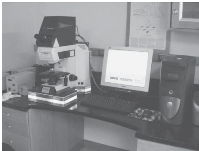
Figure 5.9 CRAIC model QDI 1000 ultraviolet–visible microspectrophotometer with Cassegrainian optics and a semiconductor array detector.
