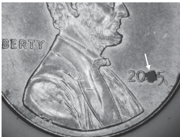
Figure 5.5 Paint fragment placed on the date of a penny for sample size perspective. (See insert for color representation.)
