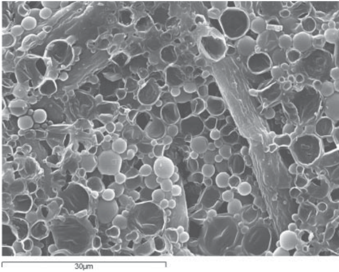
Figure 3.25 Scanning electron micrograph of the underside of a carbonless form. The microspheres range in size from 2 to 20 \mu\text{m} and are filled with normal alkanes.
