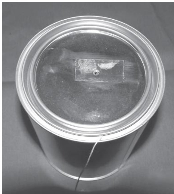
Figure 3.6 One-quart can equipped with a pressure relief device, a short strip of cellophane tape over a small hole pierced in the lid.
