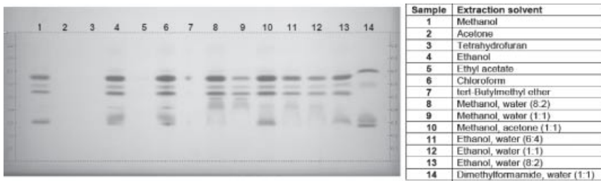
Figure 6.7 Different banding patterns based on changes to extraction solvent. (See insert for color representation.)
