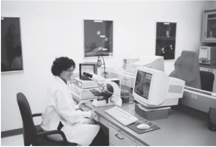
Figure 4.7 Forensic geologist using GRIM 11 instrumentation to determine the refractive index of a glass.
