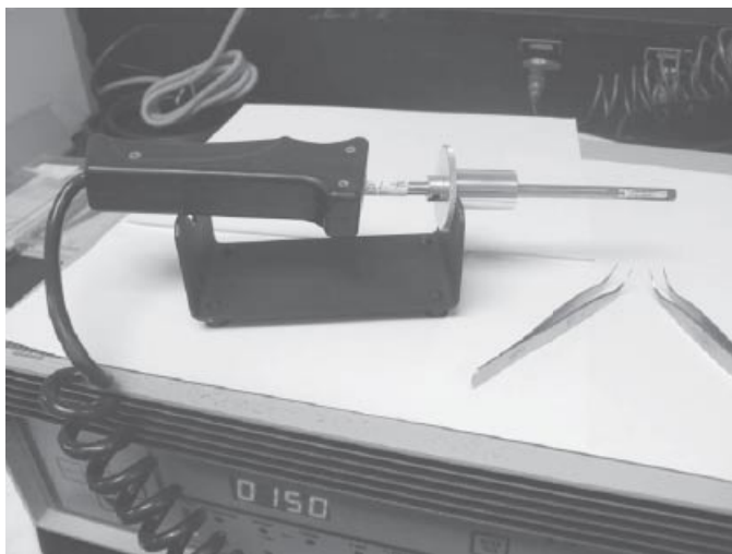
Figure 5.22 Chemical Data Systems inductively heated pyrolysis probe which inserts into the pyrolysis interface mounted on the gas chromatograph injection port.
