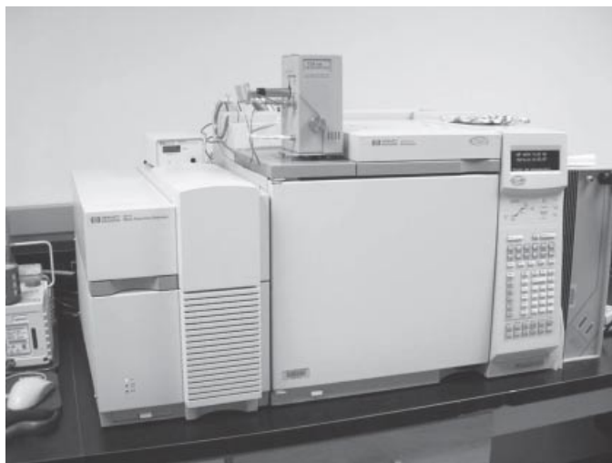
Figure 5.21 Typical pyrolysis gas chromatograph–mass spectrometer (PyGC–MS) equipped with an inductively heated pyrolysis probe, pyrolysis interface, and single capillary column having a mass selective detector (MSD).
